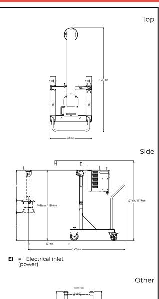
Electric Supply voltage: 380-480V/3 ph/50-60 Hz **Electrical power max:** 1.5 kW **Total Watts:** 1.5 kW
